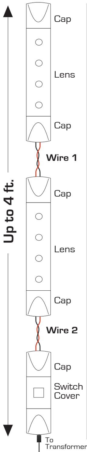
① **Measure the length you need for Wire 1 and Wire 2. Add 2" extra for the connectors. Cut using scissors. You don't need to remove the insulation.**
